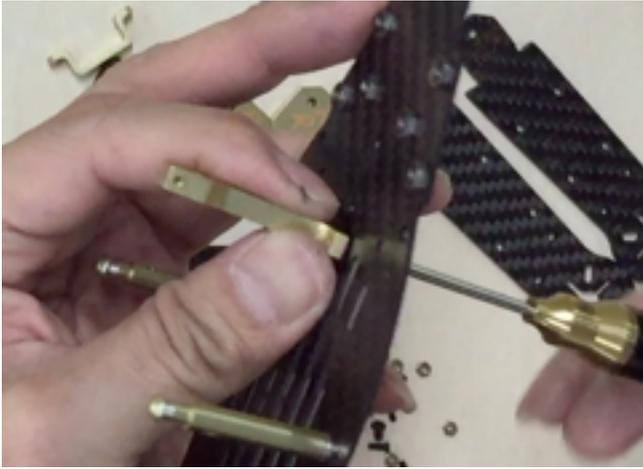
**The carbon stand needs the hex M2x4 screw at the bottom and M2x8 going through the stand and the camera ring.**
