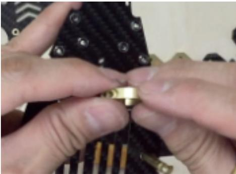
**The M2x6 also needs to lock the ring into both sides.**
