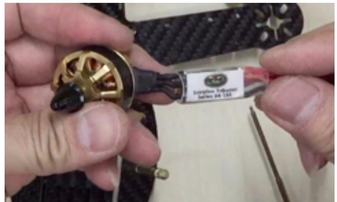
**Use M2.5x6 on the motor mounting.**
