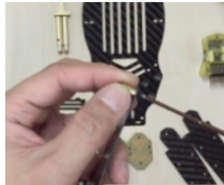
**Assemble the front spoiler set with flat M2x4 with nuts.**
