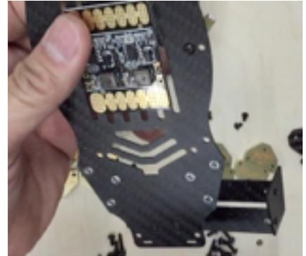
**Install the power board under the upper deck.**
